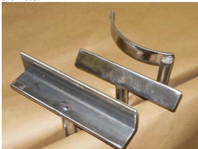
Figure 2. This photo shows the three tool rests the Author has made as described in these articles.
