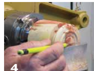
4 Use the toolrest to draw a guideline across the exact centerline of the disk. After parting off, cut the disk in half along the guideline.
