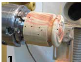
1 Turning an endgrain cylinder lets you make several card holders at once.
