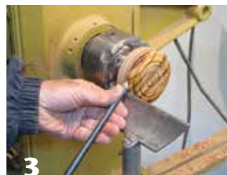
3 Make a parting cut to define the thickness of the disk and allow clearance to finish turn the bead on the rim. Here, a disk is turned from a flat board (see sidebar).
