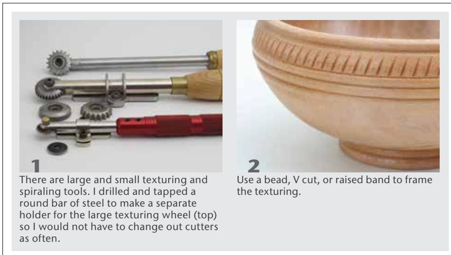
**1** There are large and small texturing and spiraling tools. I drilled and tapped a round bar of steel to make a separate holder for the large texturing wheel (top) so I would not have to change out cutters as often.
