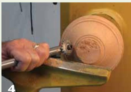
**4** Hold the texturing wheel vertical to texture the outside of a bowl. Engage cutter and lift the handle while the wood rotates at about 500 rpm. Pivot the cutter sideways to produce a line pattern instead of random dots.
