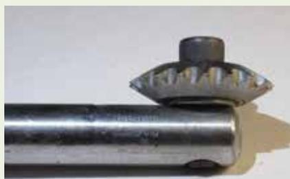
**3** A texturing wheel has teeth that come to a point. I tapped a piece of steel rod and used a cap screw to hold this texturing wheel to reduce the need to change cutters.
