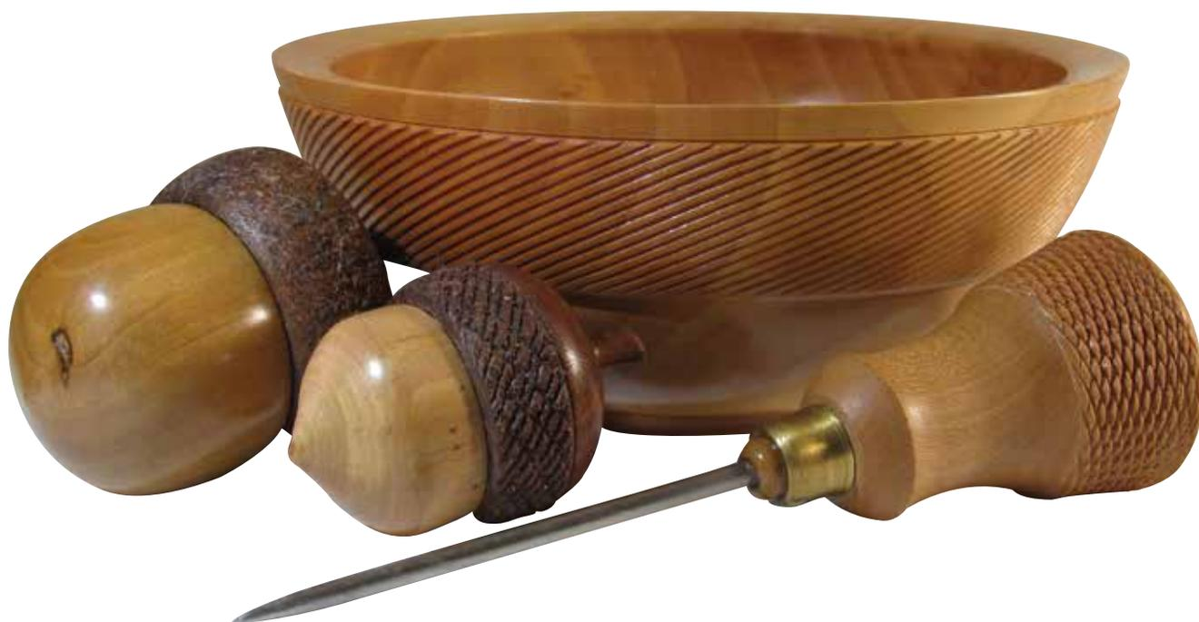
**A**dd visual and tactile appeal to bowls, platters, and spindle turnings in just moments using texturing and spiraling tools. By changing the cutter, speed, pressure, and angle, you can produce a variety of details ranging from spirals, diamonds or crosshatching, orange peel, and striations. Sorby and Crown both make texturing and spiraling tools (*Photo 1*), including minitools for delicate work.
