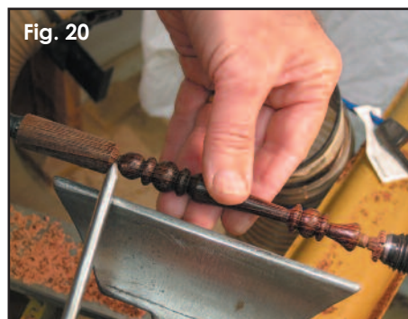
Using a skew, carefully part off the scoop handle.
