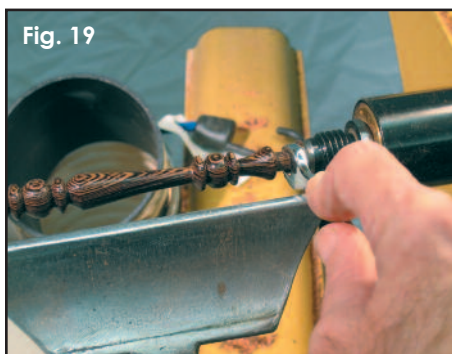
Use a 1/4" open-end box wrench to accurately size the tenon.
