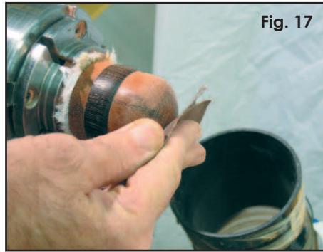
If you have a set of small jaws, use them for finishing off the bottom.
