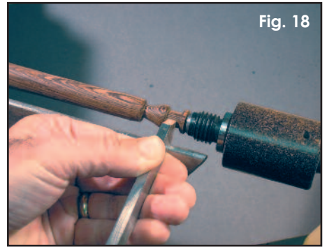
Leave room next to the handle tenon so that you can remove the hole left by the live center.
