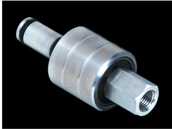
This is what I made originally. I ran across the idea of using a plastic garden hose quick disconnect. I turned a 4 ply laminated MDF outboard spinner sized the same as my PM 3520's hand wheel. This picture shows the side that slides into the spindle taken before final assembly. I built my rotary bearing adapter with a pump bearing from Lowes, part 99502-H .625 Bore, double sealed for Ace Pump found in Drawer K10, Specialty Fasteners.
