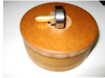
I fastened the bearing adapter with three washers in case I decide to make a better outboard spinner from Corian or something else if the MDF leaked too much. Some folks use epoxy. The small end of the garden hose fits snugly in the hand wheel and has an "O" ring that appears to seal very well. You may be able to see the white closed foam gasket on the end of the adapter that seals against the hand wheel snugly when the pump is on.
