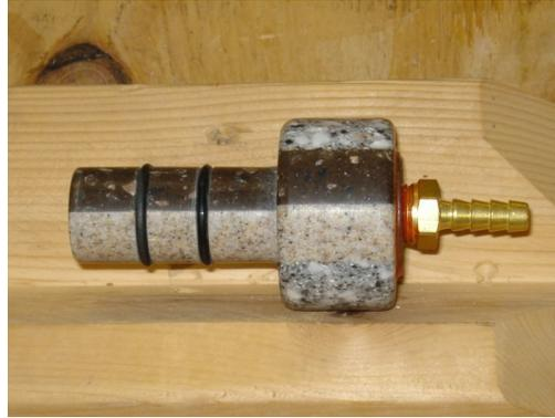
I got to meet Tom Steyer at the Southern States Symposium in 2010 and saw his rotary vacuum adapter in action. It has **two** bearings and **two** O rings.
