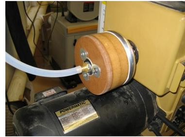
I made a holder for the rotary adapter when not in use as shown here.
