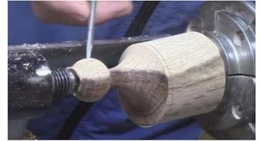
5. Take small cuts to eliminate that small nib on the top of the head left for tail stock support.
