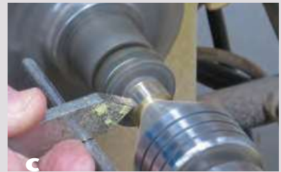
c You can use a parting tool as a scraper to remove threads or flats from brass plumbing fixtures.
