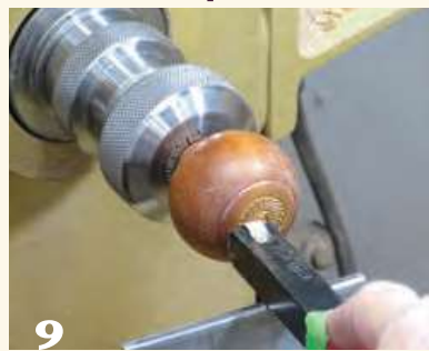
9 A knurling tool is one way to add a touch of embellishment. Note that this awl handle is held in a collet chuck, which is a good alternative to a four-jaw scroll chuck.
