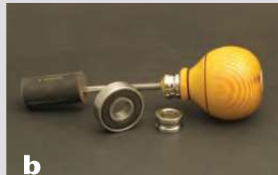
b Even an inner bearing ring can be used as a ferrule. This one came off a bandsaw.
