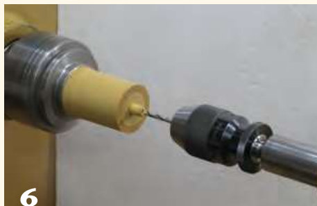
6 Drill the hole for the metal shaft.
