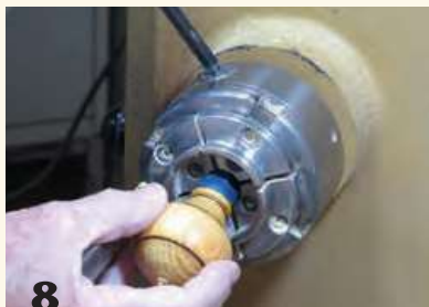
8 Reverse-chuck the handle for finishing its bottom. The bead at the top of the ferrule acts as a bearing surface against the front face of the chuck jaws.
