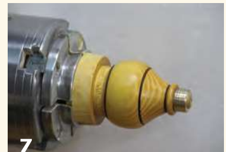
7 The handle after final shaping, with decorative burn rings added and the ferrule polished before parting off the lathe.
