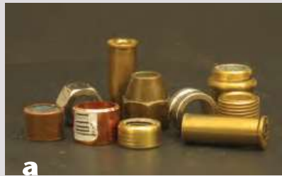
a Options for making ferrules include copper pipe, brass shell casings, and brass plumbing fittings.
