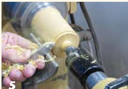
5 With the blank now mounted in a chuck, use a parting tool to shape the tenon for the ferrule.
