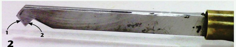
The author's shopmade dovetail recess tool, made from an old skew ½" (13mm) wide and a bit less than ¼" (6mm) thick. Surface 1 forms the bottom of the recess, and surface 2 forms the angled wall. The angle between these two edges should match the angle on the outside of your dovetail jaws (in my case, about 80°).
