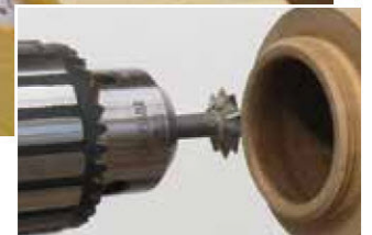
60° rotary cutter in Jacobs chuck
