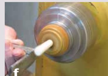
**f** Use a scraper when shaping bone on the lathe and protect your lungs from the dust.
