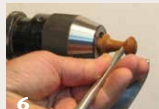
**6** You can hold an endgrain knob that you started between centers in a drill chuck. Finish shaping by taking light cuts from large to small diameter.
