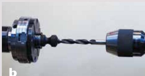
**b** Using a Jacobs chuck in the tailstock, drill a recess in the end of the knob to accept the insert material.
