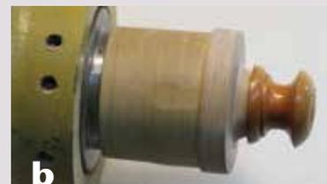
*A shopmade screw chuck assembly threaded directly onto the lathe's spindle.*
