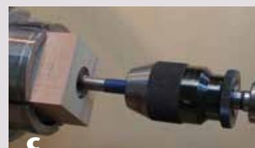
*To make a threaded block, start by drilling a hole  $\frac{1}{8}$ " smaller than your lathe's spindle diameter.*
