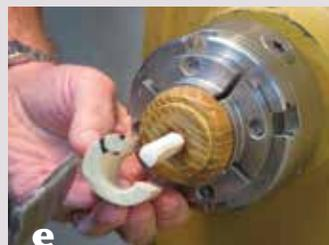
**e** Gluing a section of bone into a snug fitting hole drilled into a scrap block is an easy way to mount the material on the lathe for turning.
