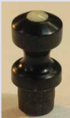
You might want to add a contrasting insert into the end of your knobs to add interest. Inserts can be of bone, vegetable ivory, or a contrasting wood species. You can easily use a plug cutter to create an insert of a contrasting wood (*Photo a*). The  $\frac{3}{8}$ " (10mm) size works well for a typical sized knob. Or simply turn a small dowel from an exotic wood and part off short sections for inserts.
