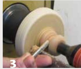
**3** Shape the bottom of the knob with the flute facing about 10 o'clock, again taking light cuts from small to large diameter.
