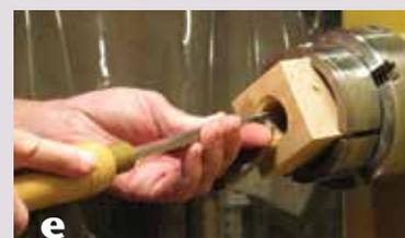
*Cut a small recess at the face of the block so it will seat properly when screwed onto the lathe's spindle.*
