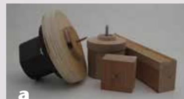
*A faceplate-mounted screw chuck (left) and one mounted on a wood block threaded to fit the lathe's spindle. Notice the faceplate-mounted screw chuck has a plywood spacer that serves the same purpose as the raised taper on the threaded block version. It serves as a sizing reference (like a pen bushing on a mandrel) when turning the base of a knob and provides clearance for shaping the bottom section of a knob.*
