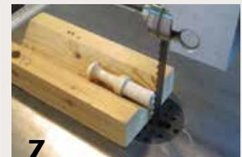
**7** Use a shopmade V-block to safely cut a slot for a wedge at the bandsaw.
