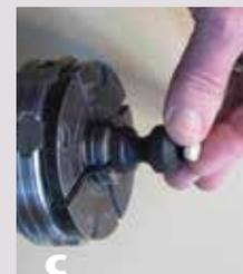
**c** The insert material should initially stand proud of the knob surface so it can be turned and sanded flush later.
