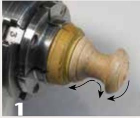
**1** Proper direction of cut for the smoothest surface when the workpiece is mounted in facegrain orientation.
