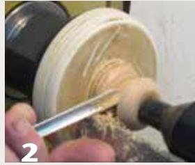
**2** Take light cuts with a spindle gouge with the flute facing the 2 o'clock position, cutting from small to large diameter if the workpiece is mounted in facegrain orientation.
