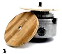
Use a plywood spacer when a smaller-depth hole is required.
