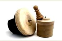
Smaller-size shopmade screw chucks provide fast and easy mounting of small projects such as chessmen (right). Use a lag bolt if more support is needed, as shown in the example on the left that uses a faceplate and a scrap of plywood.
