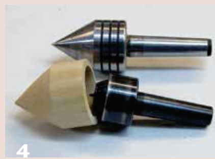
4 If you do not have a 60-degree cone center, turn one to fit over your existing live center.
