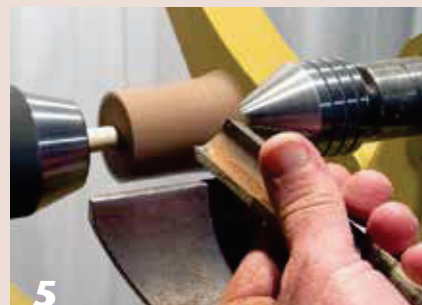
5 The initial roughing of the wood can be done using a spindle-roughing gouge.
