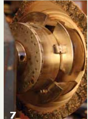
**7** Deeper/longer jaws are needed for natural-edged bowls when remounting them to complete the outside profile.
