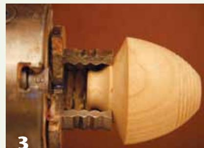
3 The detail on the shoulder of this small vase provides a groove on which the dovetail jaws grip.
