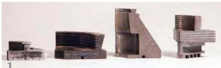
1 Only the tallest jaw (second from right) has an inner rim that will grip around a foot without leaving a mark.
