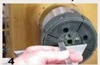
It is easy to turn nylon jaws to your needs using regular turning tools. Here, a negative-rake scraper forms a straight-sided recess.
