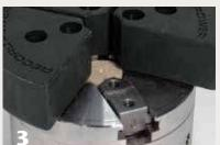
Before turning the nylon jaws to shape, clamp a dowel in the jaw slides.
